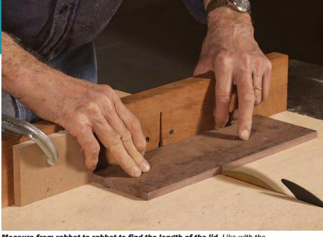
**Measure from rabbet to rabbet to find the length of the lid.** Like with the plywood bottom, Stowe sets his fixed stop to this dimension when cutting the solidwood top to length (above).
