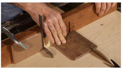
Add a shim between the stop and the spacer when cutting the solid-wood top to width. The shim accounts for the seasonal expansion of solid wood while still allowing you to use the same spacer and stop.
