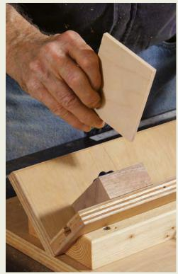
Add the removable spacer next to the fixed stop and cut the next series of splines. Stowe uses a square of ½-in. Baltic-birch plywood, allowing for regular, reliable spacing between the splines without disturbing your fixed stop.
