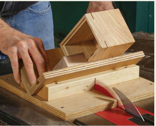
**Cut the first series of splines.** Stowe uses a thin-kerf ripping blade. It makes for splines with a lighter look than standard 1/6-in.-thick blades, and its flat rip teeth leave a square cut, perfect for the splines to fit without gaps.
