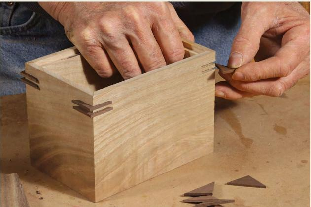
Glue in the splines, then trim them flush. Because the bottom is plywood glued in place, the box needs reinforcing splines only at the top. Using triangles of wood for the splines minimizes waste.
