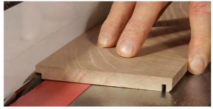
The sides' blanks get a groove toward the bottom edge and a rabbet at the top. The groove captures the bottom, and the rabbet recesses the lift-off lid.
