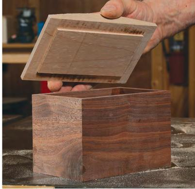
A rabbet runs all around. Because the top was cut to width with a spacer and shim, you can use the same rabbet setup on all four sides of the top's bottom face. If you didn't use the shim, the rabbet would have to be wider along the sides, reducing machine efficiency.
