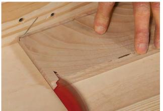
Miter one end of the blank using a sled. This cut establishes the box's first corner. Stowe places the outside face down on the dedicated miter sled, whose zero-clearance kerf lets him both align the cut easily and limit blowout.
