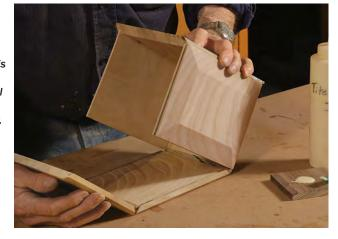
Like with the other lids, make this one by using a fixed stop when cutting it to length and the removable spacer and shim when cutting it to width. To cut the grooves, I head to the router table and employ a slot-cutting bit. Use the same setup for both the box sides and the lid. To keep the lid's grooves from weakening the workpiece too much, I like the stock to be at least 3/8 in. thick.
