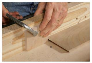
Set the fixed stop, flip the workpiece, slide it up to the stop, and cut. The stock's inside face is down for this cut, and the fixed stop is set to the length of the long side. The stop remains in place until you've cut all the miters for each box.
