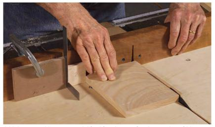
Add the removable spacer and thin shim when cutting the panel to width. Because wood expands and contracts across its width, Stowe adds the shim to size the panel slightly narrower to keep the wood from pressing against the box sides during humid months.
