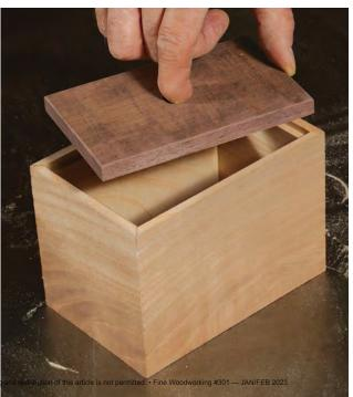
Drill a finger hole for easy lift-off. If you can't get a good grip on the lid's edges because it sits too deeply in the rabbets, drill a hole in the middle for a low-profile lift.
