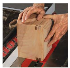
Start cutting the lid free by ripping along the box's short sides. Hold the box tight to the table and the fence. At layout, space the spline slots to allow room for this kerf.
