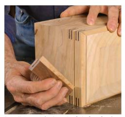
Install spacers in those kerfs before freeing the lid by ripping the long sides. The spacers, held in place with rubber bands, keep the kerfs from closing and pinching the blade. They also prevent the lid from falling away prematurely and possibly getting damaged. Stowe reattaches the lid with hinges.
