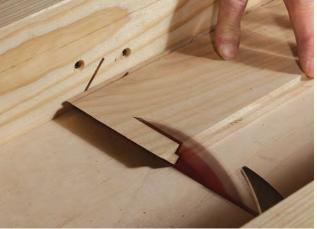
Make a short cut at that mitered end. After completing the first box side (above), flip the rest of the blank outside face down and trim off the end in a clean miter. Cut as little as possible to maintain continuous grain.
