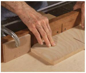
**Crosscut the panel to length against a fixed stop.** Set the fixed stop to a snug fit between the short ends' grooves, since wood does not move much along its length.
