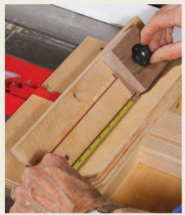
Set the stop on a splining sled. Stowe makes a lot of boxes and has a souped-up sled for cutting slots for splines. Even with a simpler setup, the principle is the same: Lock down a stop for the initial slot; add spacers for subsequent ones.
