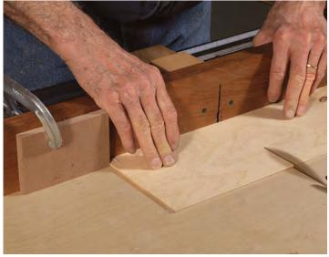
Use the removable spacer to cut the bottom panel to width. The box's bottom is plywood, so you don't have to account for wood movement. Instead, you want a good allaround fit for glue.
